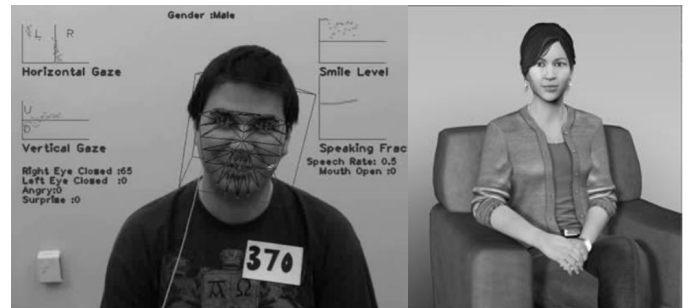
Figure 1: This is a side by side view of a participant interacting with Ellie, the SimSensei agent (seen on the right side). On the left side, we see the participant being tracked in real-time by MultiSense, the multimodal perception system used in SimSensei. The participant’s tracked state informs the automatic system and enhances the interaction.
